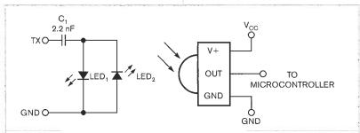
Figure 1 By sending appropriate hex values to a PC's serial port, this circuit generates precise bursts of 38.4-kHz data.
